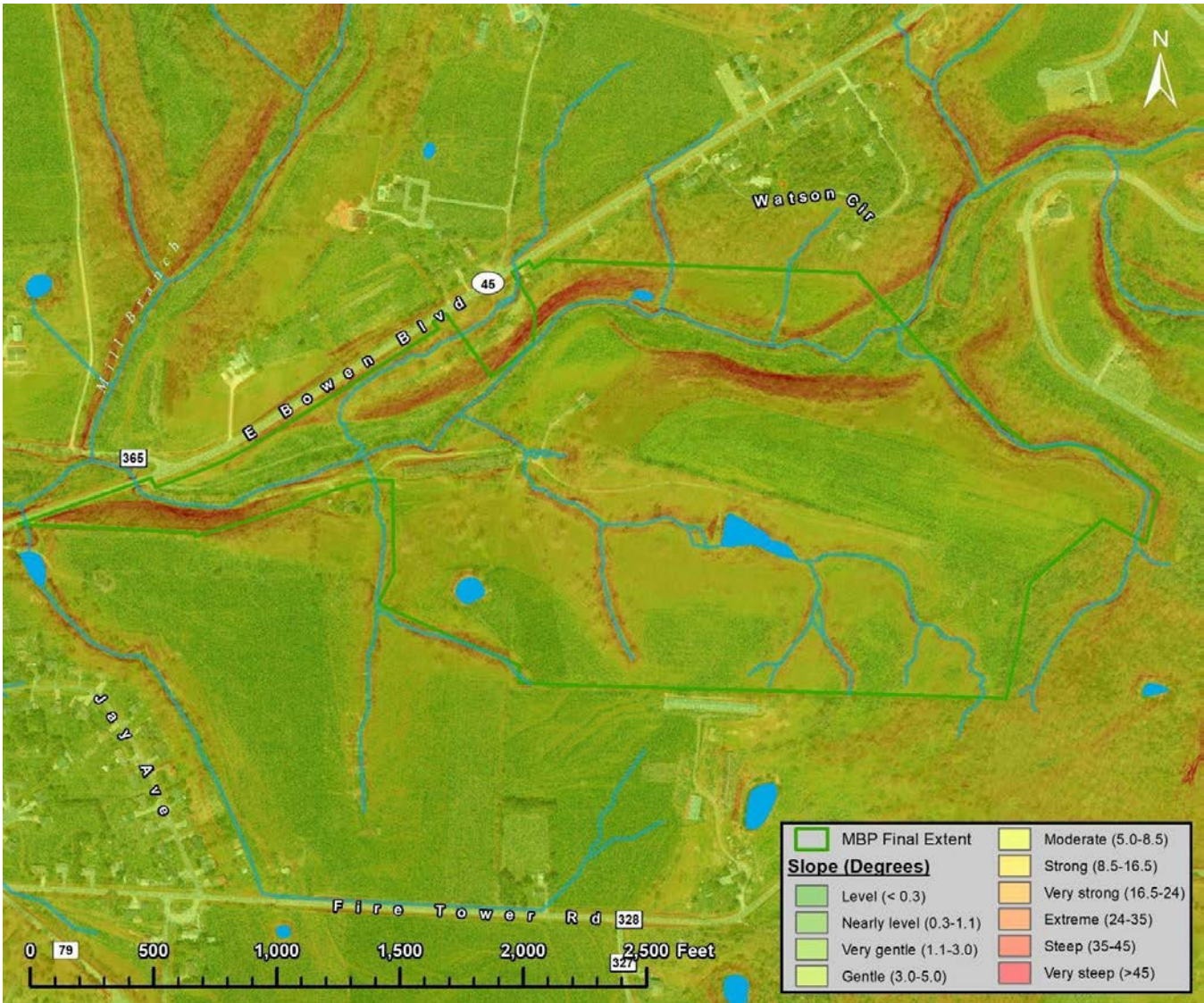
Figure 14: Slope map of Mill Branch Park. Slopes greater than 10 degrees are considered undesirable for casual walking, and all paths should ascend slopes at an angle to avoid gully formation.
