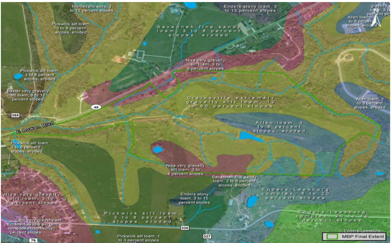
Figure 16: Soil features of Mill Branch Park. Gravelly soils (red and yellow) are very permeable, tending to be great at filtering stormwater and recharging groundwater but also prone to drying out quickly and favoring drought-tolerant plant species. More fertile silt-loam soils (blue, green) tend to recharge groundwater more slowly but also support more vegetation due to their sponge-like ability to hold moisture.
